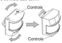
If the sensor pops out of the ball joint, loosen the clamp screw and push the sensor back into the ball joint. Tighten the clamp screw when done.
